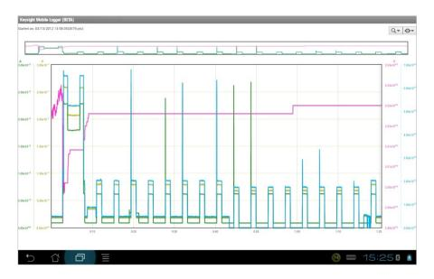
Figure 2. Voltage, current, and power trend logging with Keysight Mobile Logger app
